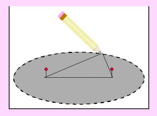
The place where each pin is is a focus (the plural of which is foci). The sum of the distances from the ellipse to these points stays the same because it is the length of the string.
